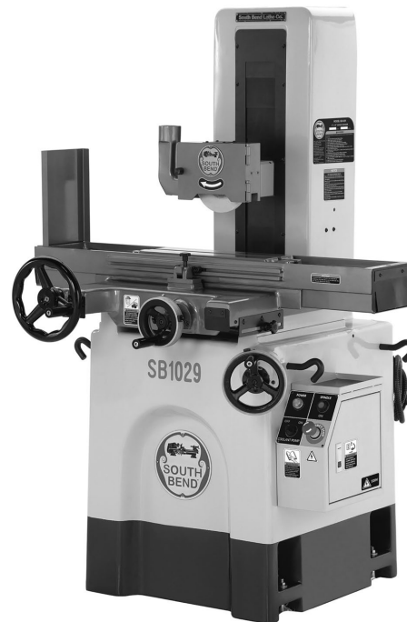
■ Figure 1-9 A surface grinder is used to grind flat surfaces. (Source: South Bend Lathe Co.)
