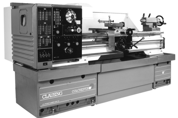
■ Figure 1-6 An engine lathe is used to produce round work. (Courtesy of Clausing Industrial, Inc.)
