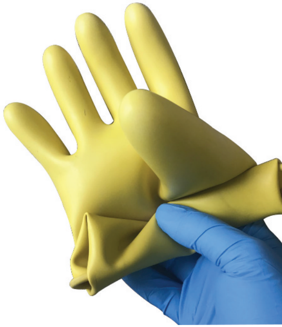
FIGURE 1-7 The glove is rolled up on the open end to check for air pressure and any air leakage.
