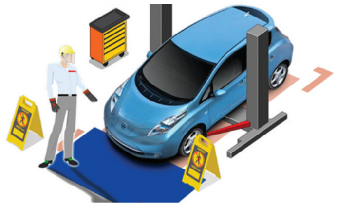
FIGURE 1-3 A clearly defined safety zone needs to be established in the area where a hybrid or electric vehicle is being repaired.
