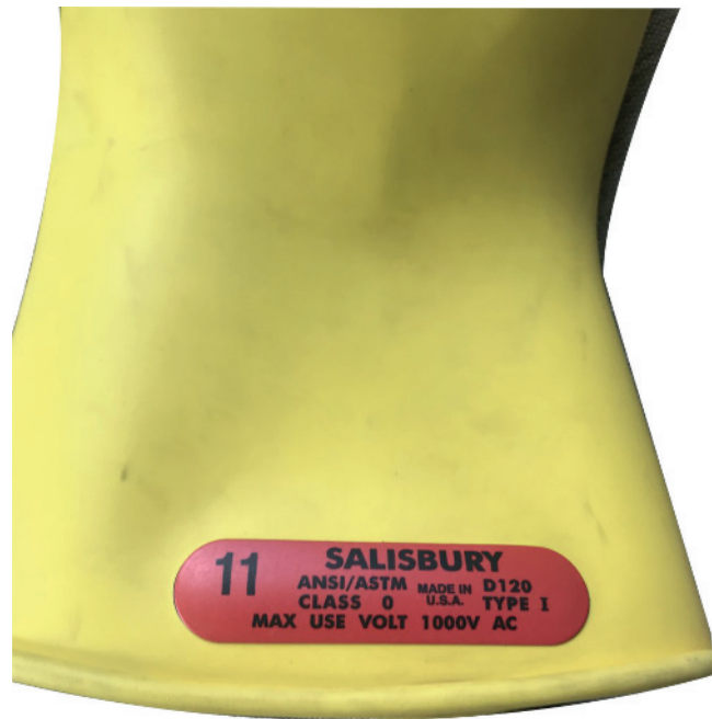
FIGURE 1-6 The gloves should be clearly marked indicating that they are class “0” and rated for 1,000 volts.
