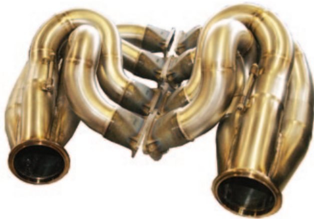
FIGURE 1-16 Formula 1 racecar exhaust manifold constructed from stainless steel tubing.
