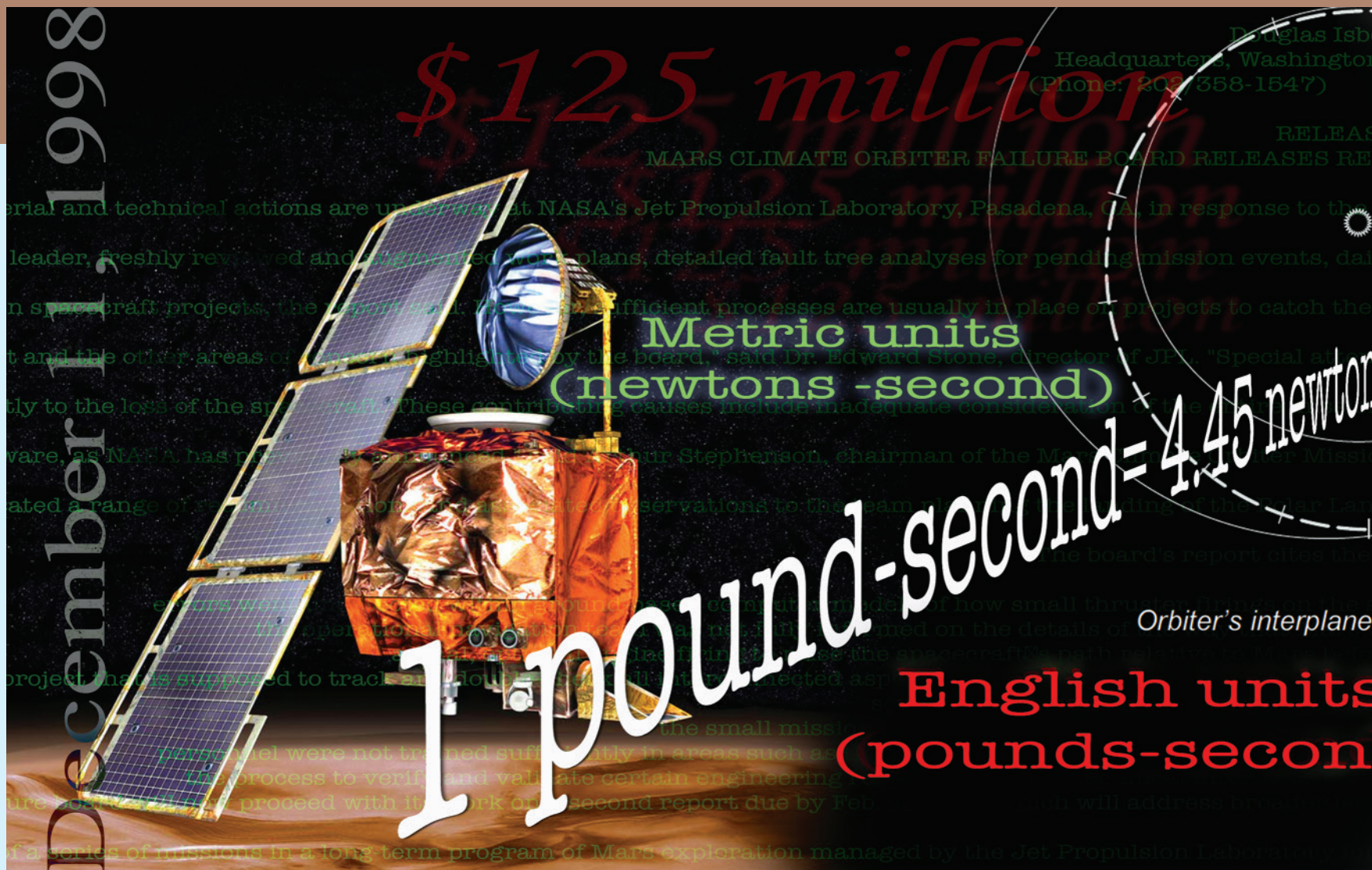
The $125 million Mars Climate Orbiter was lost in the Martian atmosphere in 1999 because of a unit mix-up.
