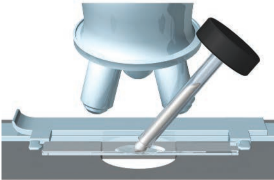
(b) Place a drop of immersion oil in the center of the slide.
