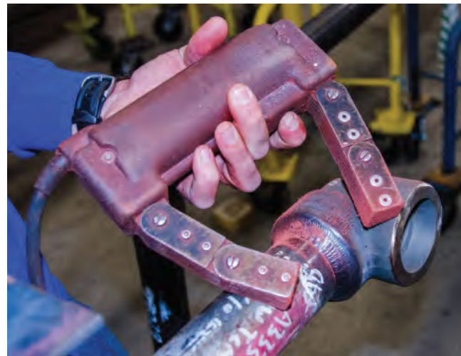
Fig. 1-8 Using a method of weld inspection known as magnetic-particle testing in pipe fabrication. This non-destructive method followed by radiograph and/or ultrasonic testing assures weld soundness for critical pipe welds. Mark A. Dierker/McGraw Hill
