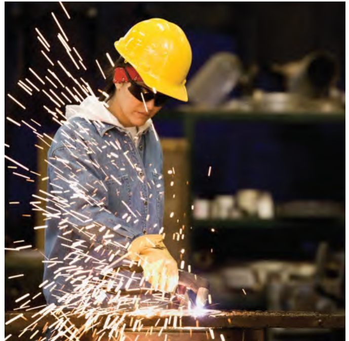
Fig. 1-5 Welding is generally considered a nontraditional occupation for women. However, it can be a very lucrative and in-demand skill for those women choosing this career path. A procedure is being used setting up a plasma arc gouging operation. Andersen Ross/The Image Bank/Getty Images
