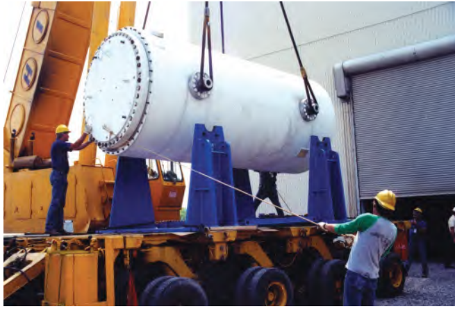
Fig. 1-9 Workers using a crane to lift a cask filled with highly radioactive fuel bundles at a Hanford, Washington, nuclear facility. The construction of this type of vessel relies heavily upon welding. U.S. Department of Energy, The Monroe Evening News/AP Images
