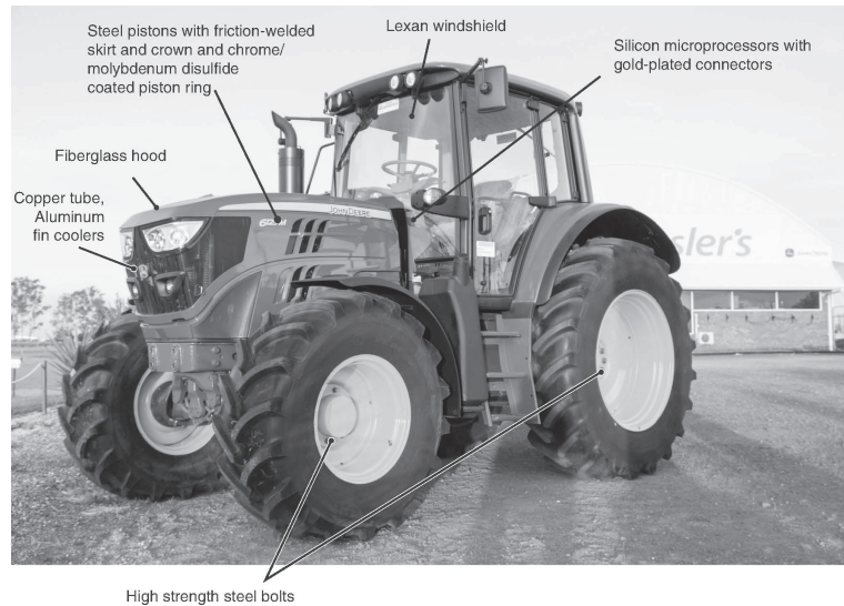
FIGURE 1.1 John Deere tractor showing the variety of materials and processes incorporated. Source: Shutterstock/Nils Versemann.
