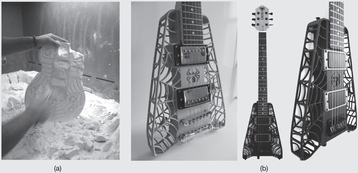
FIGURE 1.4 Guitars produced through additive manufacturing. (a) Spider design being removed from a powder bed. Note that the support material, or cake , has some strength and needs to be carefully removed; (b) finished Spider guitars. Source: Courtesy of O. Diegel, Massey University, New Zealand.
